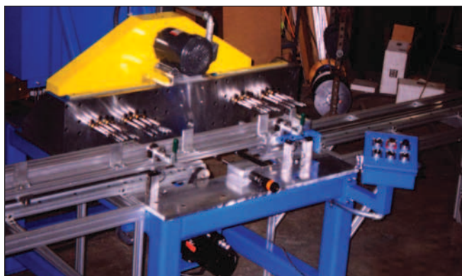
Door frame drilling jig. With LoPro's precise travel and fast acceleration, exact placement of holes for production door frames is easy and repeatable every time.
